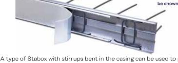
A type of Stabox with stirrups bent in the casing can be used to produce a reinforced concrete corbel. The stirrups can be bent in accordance with the models D4, D6 and D7 below.
