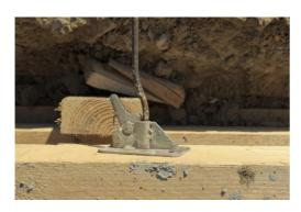
The rapid clamp with spring, consisting of an eccentric axis and an internal spring, allows formworks to be clamped on bars with a diameter of 5 to 10 mm.
