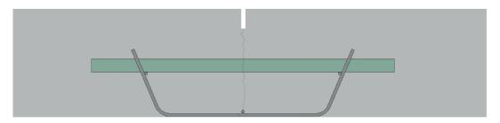
The standard round dowels are made of mild steel with 25mm diameter and 600mm length. They are protected by a thick epoxy coating that is resistant to salt spray tests.
